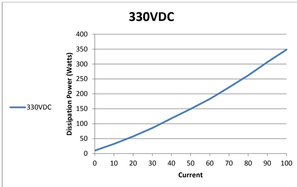
Figure 3: Power Dissipation for “400V” types
