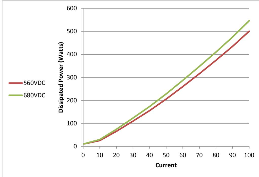
Figure 2: Power Dissipation for “800V” types
