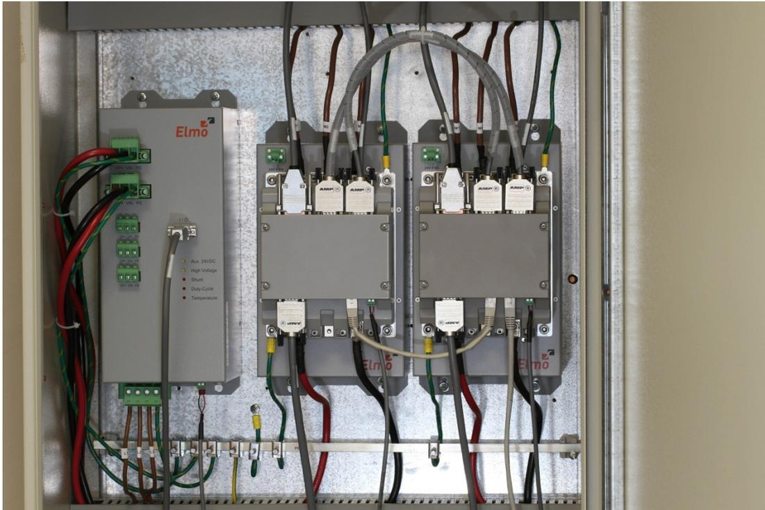
**Figure 7: Typical Two 60kW Gold-Drum Servo Drives, Powered by Elmo TAM-100/480 (Power Supply for Servo Applications), in the Elmo Gantry Configuration**
